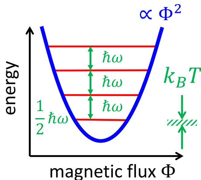
Microwave frequency circuits:  $\omega/2\pi \sim 5 - 10$  GHz
