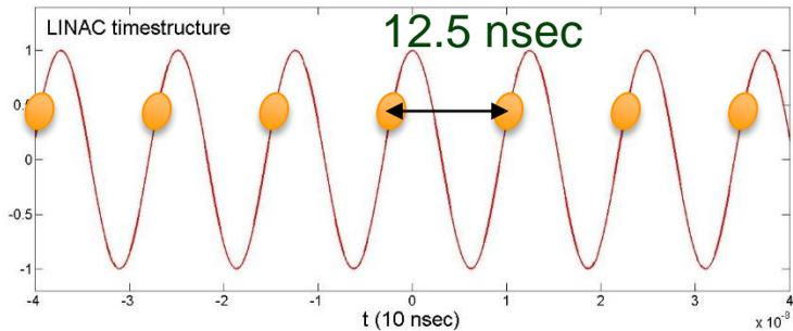
With low frequency prebuncher, 16 MHz
