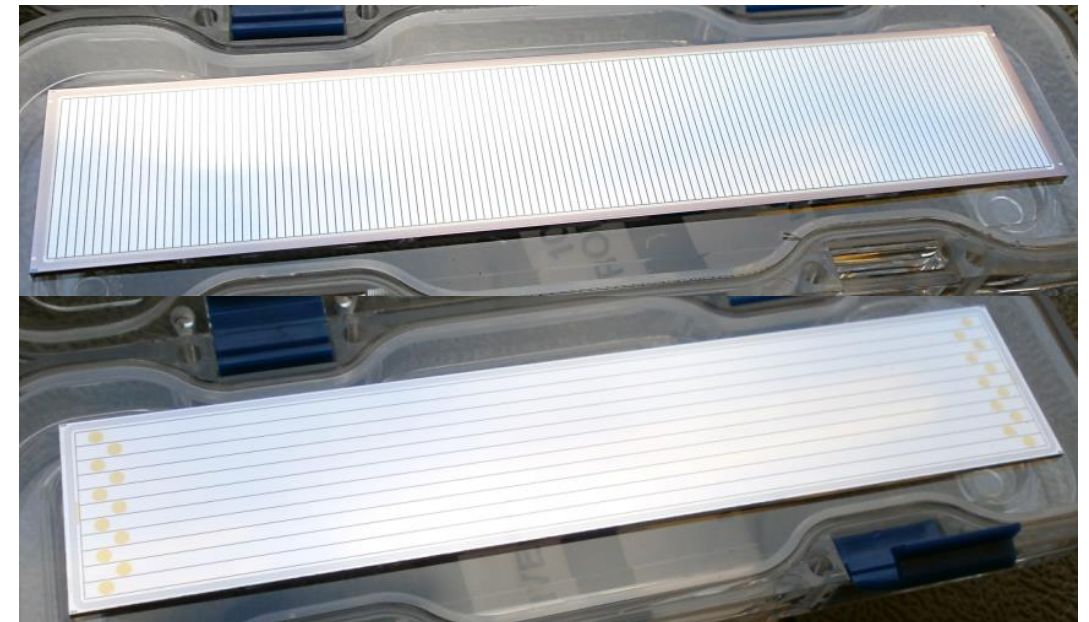
Figure 2 Photographs of double-sided silicon strip detectors. The top and bottom photographs show the full junction and ohmic sides, respectively.
