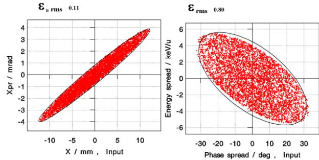
Figure 6:  $U^{4+}$  input particle distribution used for simulations of the new 108 MHz pre-stripper section starting at the HSI exit at 1.4 MeV/u.
