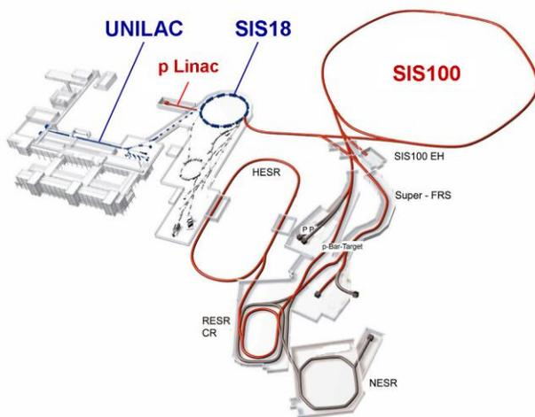
Figure 1: Sketch of the FAIR facility [1]. The existing GSI accelerators (indicated in blue) with the UNILAC heavy-ion linac and the SIS18 synchrotron will serve as injection chain for the new SIS100.
