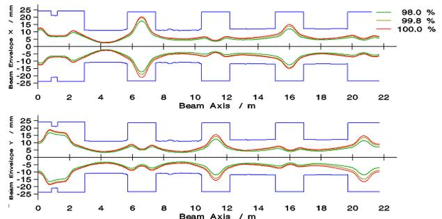
Figure 7: Transverse beam envelopes in the horizontal (top) and in the vertical plane (bottom) along the new 108 MHz pre-stripper section starting at the HSI exit.
