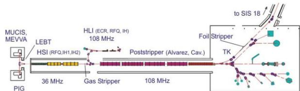
Figure 2: Layout of the present heavy-ion UNILAC accelerator at GSI and low-energy experimental area.
