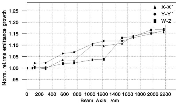
Figure 8: Relative rms emittance growth from HSI exit down to the stripper position for a 20 mA U<sup>4+</sup> beam.
