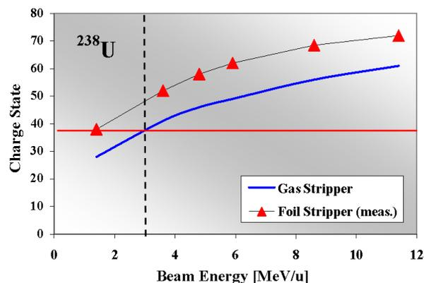
Figure 4: Main uranium charge state after stripping at different stripper materials as function of beam energy.
