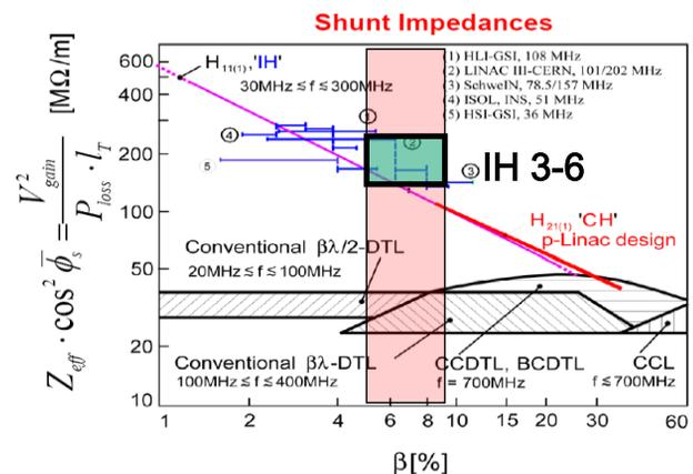
Figure 10: Estimated effective shunt impedances of the new 108 MHz pre-stripper IH cavities as compared to conventional structures and further H-mode cavities.
