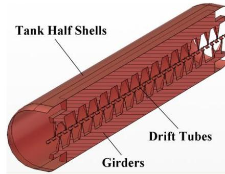
Figure 9: Simulation model of the first 108 MHz IH cavity of the presented HE linac study.
