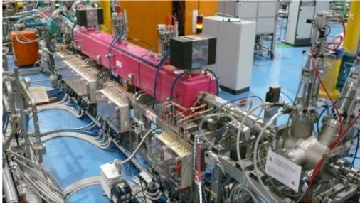
Figure 2: RFQ and IH structure in synchrotron room.
