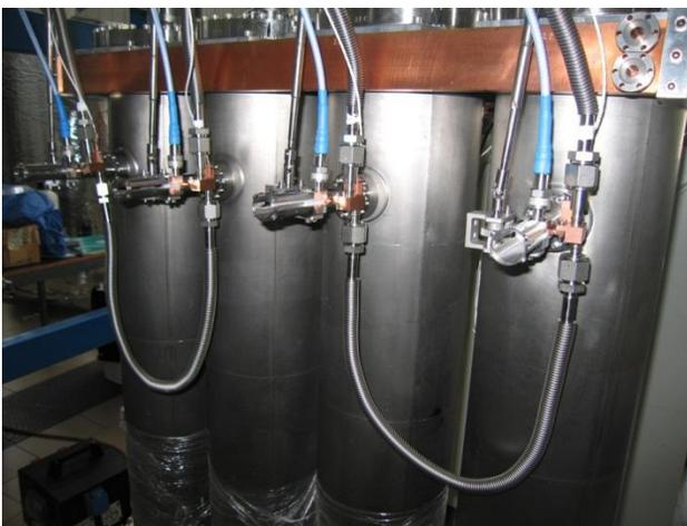
Fig. 3: Photo of the N-cooling scheme of full Nb 80 MHz QWRs of ALPI.
