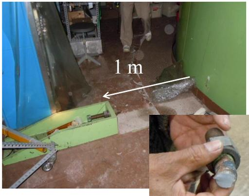
Figure 3: Broken shock prevention device for the accelerator tank at the 7th floor. Anchor bolts of 1 inch in diameter for the shock prevention device were severed by the shock of the earthquake.
