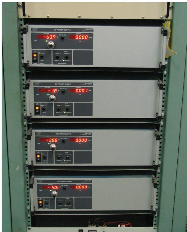
Figure 1: Bipolar power supplies block with continuous zero crossing capability for an electrostatic deflection system
