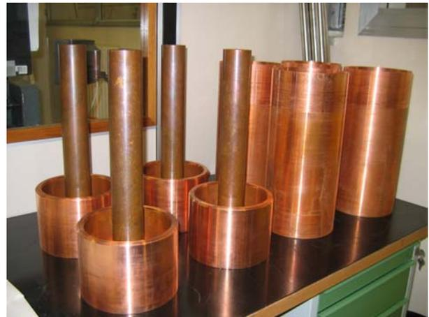
Figure 3: OFHC Cu cavity parts before vacuum brazing.
