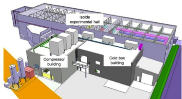
Figure 3: New HIE-ISOLDE buildings.
