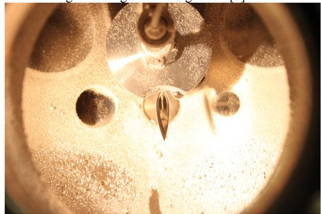
Figure 3: Liquid lithium film established at ANL.
