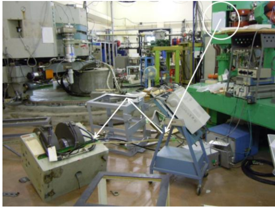
Figure 8: Dropped \beta -NMR experimental magnet at the 1-F beam course of the 1st floor.
