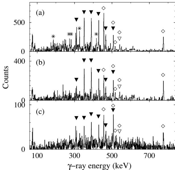
**Fig. 1.** (a) Spectrum created by double-gating on all pairs of  $\gamma$ -rays in the list (309.7 keV, 350.3 keV, 388.8 keV, 427.9 keV, 466.0 keV). (b) Spectrum created by double-gating on clean pairs only. (c) Triple-gated spectrum, created using the same gate list as (a). See text for details.
