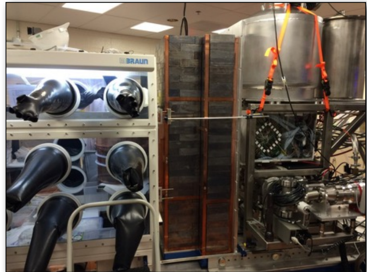
Module mated to the glovebox for string installation
