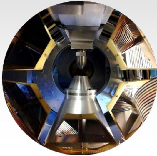
JENSA Gas-jet target – windowless Gas target (e.g. H,  $^2\text{He}$ ,  $^3\text{He}$ ,  $^4\text{He}$ ) for low-energy reactions in astrophysics
