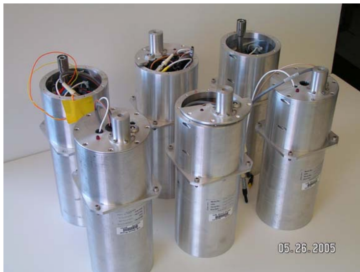
Fig. I-82. Six of the large germanium detectors obtained from the DOE Remote Sensing Laboratory for refurbishment. The crystals are being remounted in liquid-nitrogen cooled cryostats for laboratory use.
