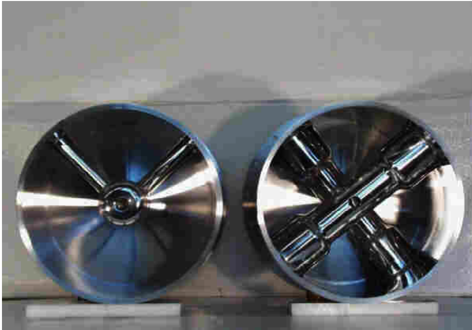
Figure III-2. Aluminum models of the 172 MHz lollipop cavity and 345 MHz spoke cavity being developed for the RIA driver linac.
