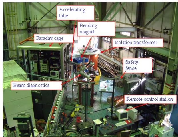
Figure 1: General view of the injector.
