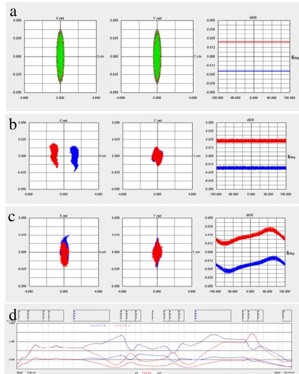
Figure 5: Beam phase space plots and envelopes in the LEBT. a – input beam; b – downstream of the slits; c – downstream of the MHB; d – full and RMS envelopes for Bi<sup>24+</sup> and Bi<sup>25+</sup> dual charge-state beam.
