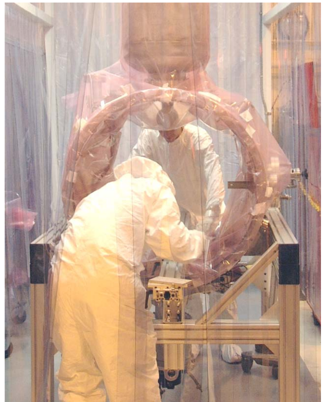
Figure 4: Clean room assembly of a horizontal test cryostat for the two-cell spoke cavity. The system incorporates separate cavity and cryostat vacuum systems to enhance cleanliness.
