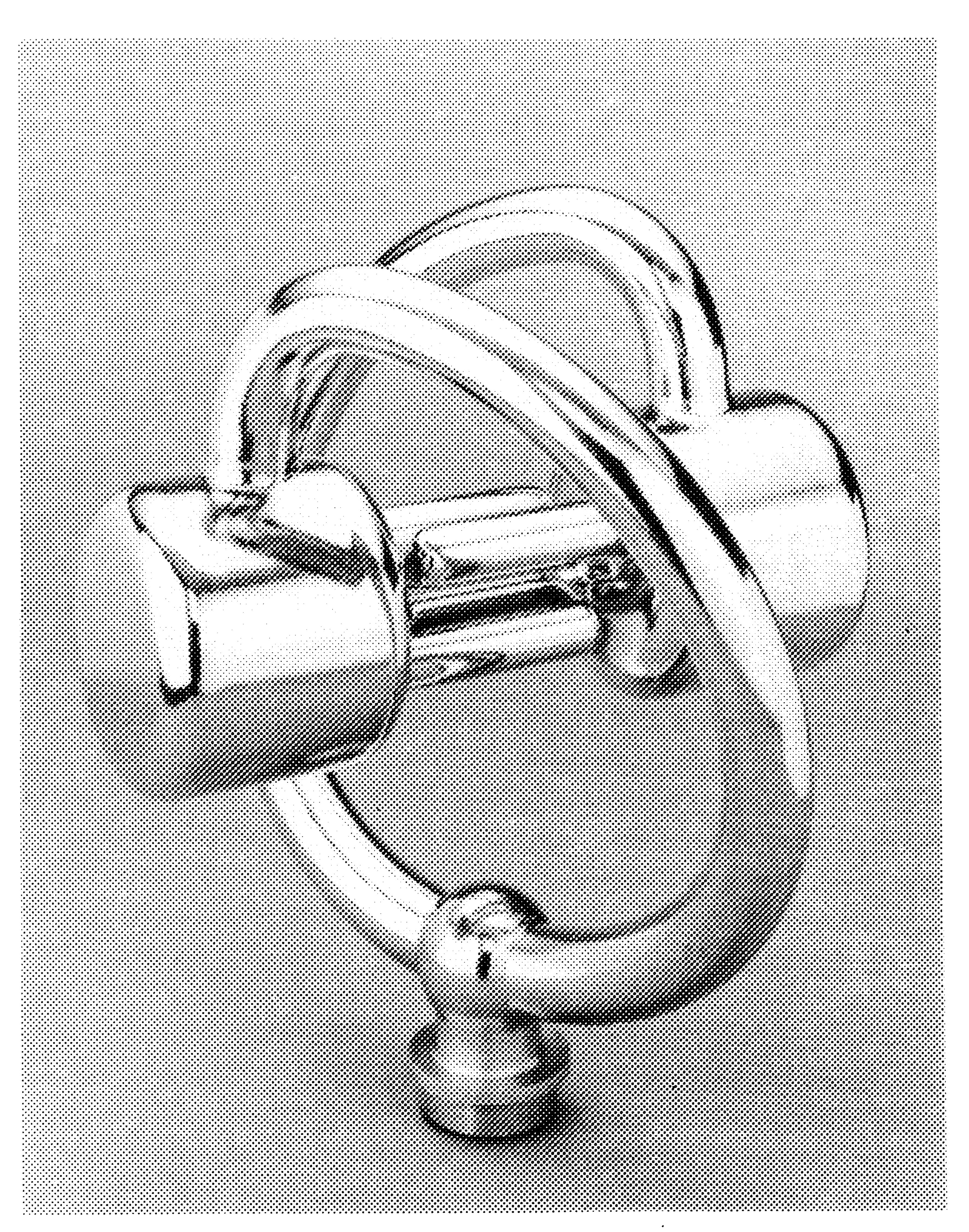
Fig. 1. Niobium split-ring assembly with RFQ vanes prior to being welding into the outer housing.
