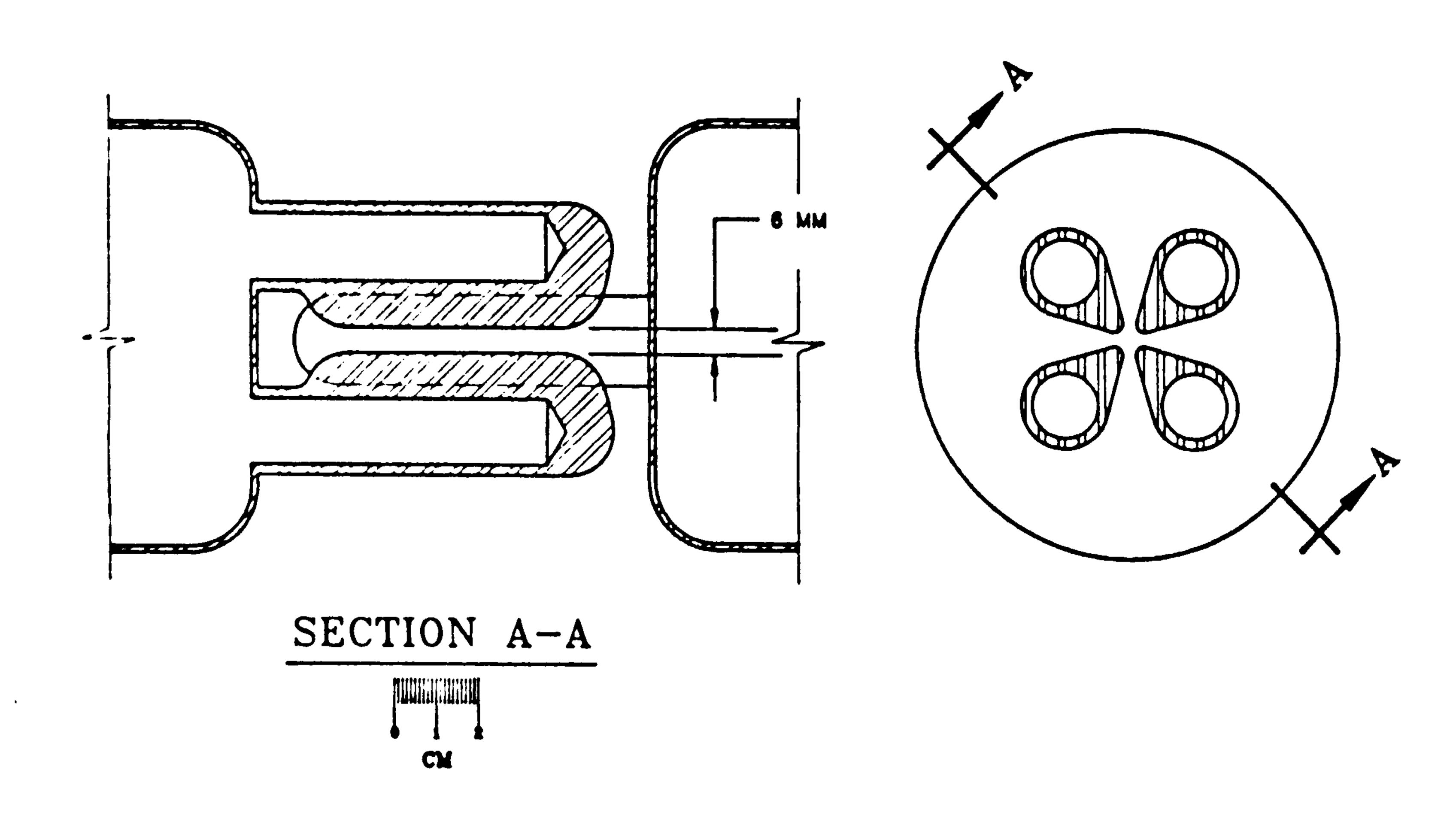
Fig. 2. Geometry of the vanes generating the rf quadrupole fields.
