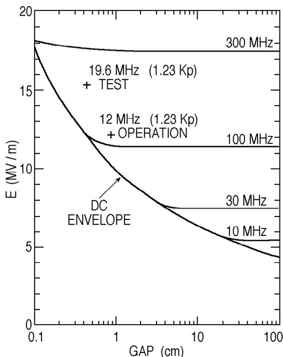
Fig. 3. Electric field limits in the Kilpatrick model, showing both gap and frequency dependence. The model test results and extrapolation are discussed in the text.
