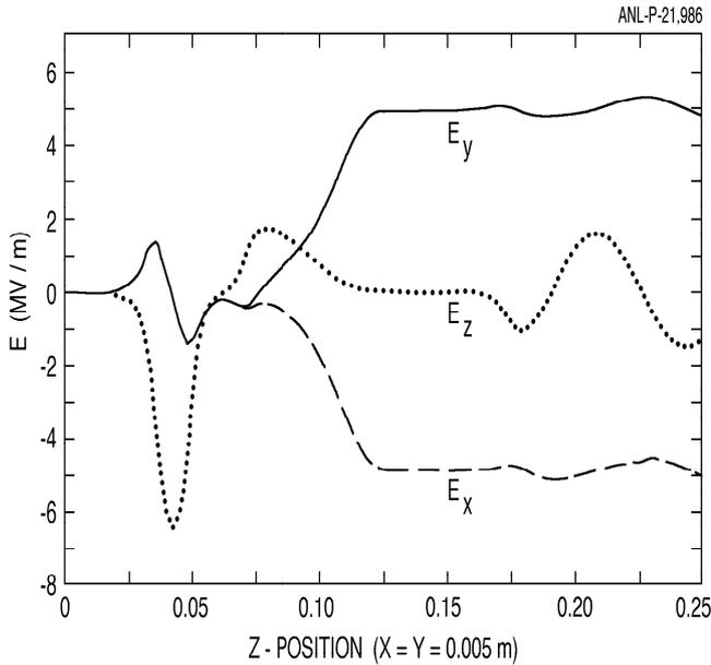
Fig. 1. Electric fields at the entrance of the RFQ, from TOSCA. A drift-tube 20 mm long, centered at  $z = .06$  meters, is tied to the high-voltage vane pair.
