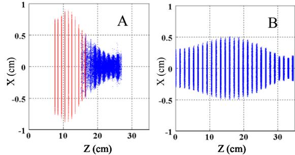
Figure 4: Envelopes in conventional (A) and modified (B) RFQ entrance radial matcher.
