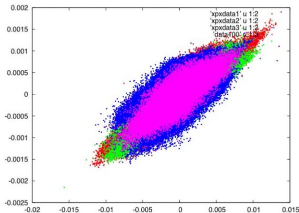
Figure 1: Transverse phase-space plot ( $x$  vs  $p_x$ ) of 10M particle simulation for three-charge-state uranium beam at the exit of linac for the MSU RIA design. As described in the text, the plotting algorithm displays all the halo particles. The dense central region is obtained by plotting every 100<sup>th</sup> particle.
