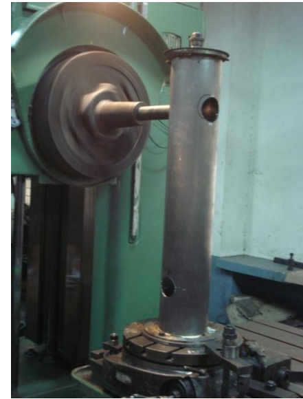
Outer Housing - boring of Coupling and Beam Ports
