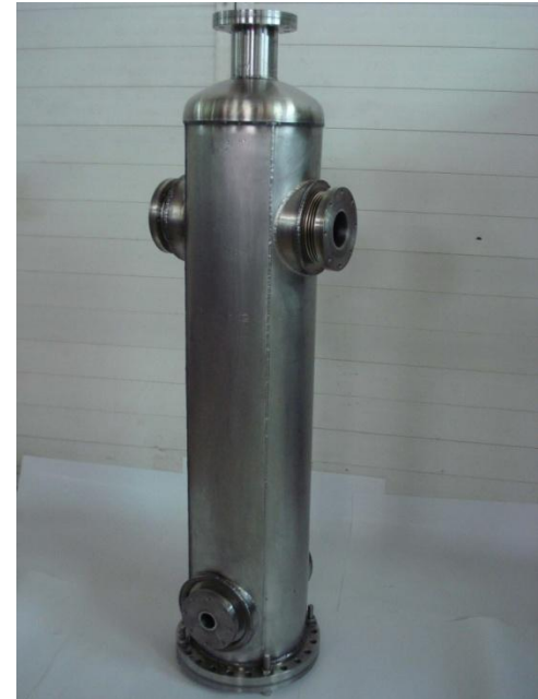
Prototype Low Beta Resonator complete with the outer Stainless Steel vessel (May 2012).
