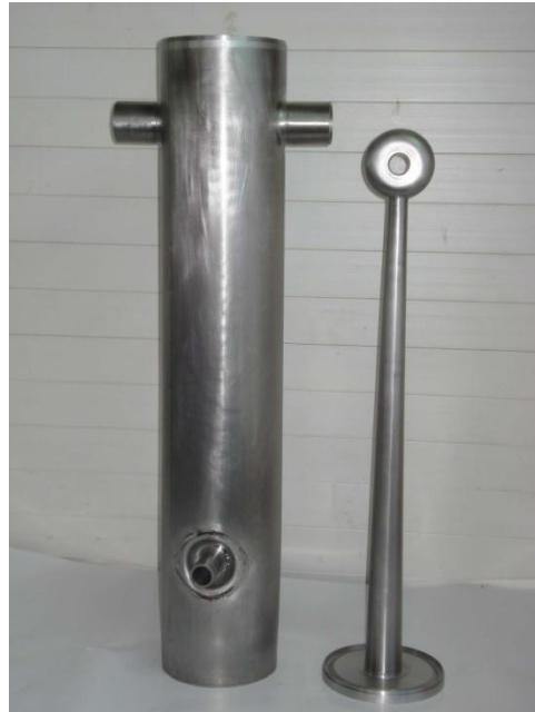
The two major sub-assemblies of the niobium resonator - Outer Housing (left) and Central Conductor with Top Flange (right).
