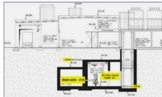
Machine underground (beam axis = - 8m)
