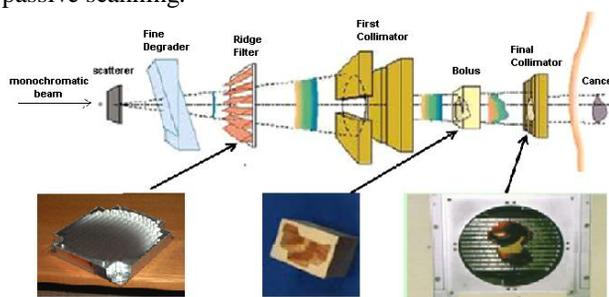
Figure 2: Scheme of a passive scanning.
