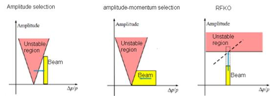
Figure 7: Steinbech diagrams of the three methods to put the beam in resonance.
