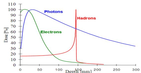
Figure 1: Bragg peaks in the case of photons, electrons and hadrons□
