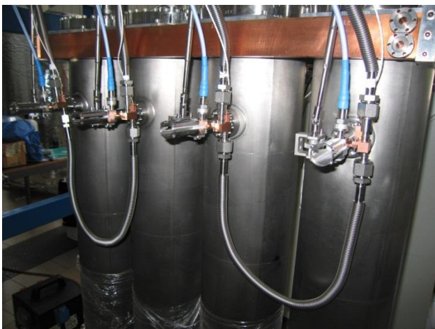
Fig. 3: Photo of the N-cooling scheme of full Nb 80 MHz QWRs of ALPI.
