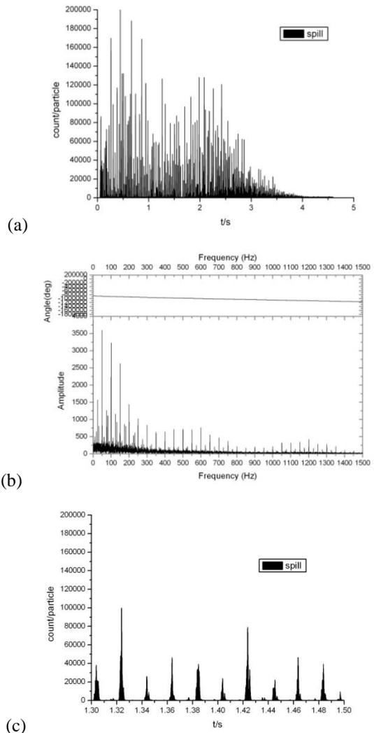
Figure 1: Spill in normal mode (sample rate is 10 kHz). (a) Structure of one spill, (b) The FFT of one spill, (c) Detailed spill structure in 1.3s-1.5s.
