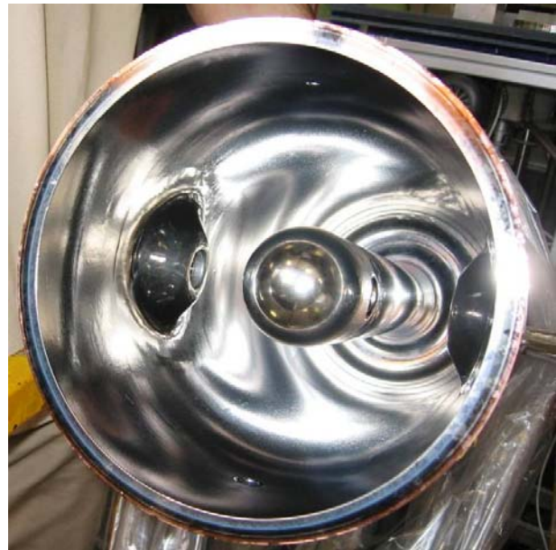
Figure 5: New medium \beta cavity after being sputtered and before being closed by its bottom plate.
