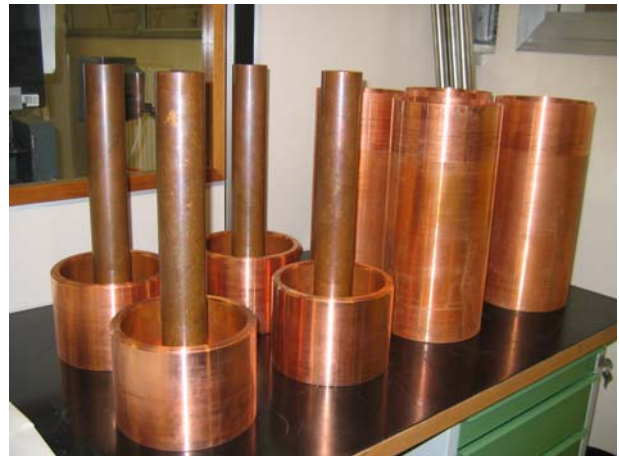
Figure 3: OFHC Cu cavity parts before vacuum brazing.
