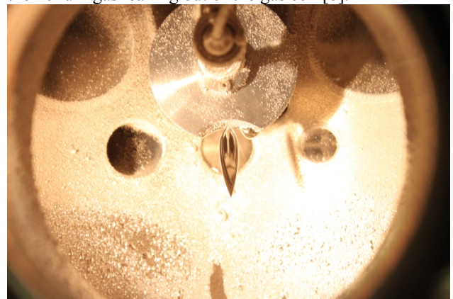
Figure 3: Liquid lithium film established at ANL.
