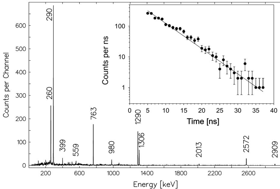
FIG. 1. A  $\gamma$ -ray spectrum, showing  $\gamma$  rays coincident with the 1290 or 763 keV transitions. Additional constraints are simultaneous detection of one  $\alpha$  particle, one proton, and at least one neutron and the detection of all  $\gamma$  rays within a time window between 9 and 38 ns after the reaction. The inset shows a time spectrum of the 2572 keV  $\gamma$  ray.
