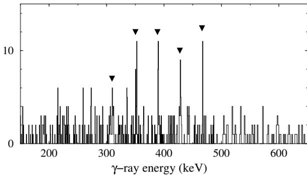
**Fig. 5.** Spectrum created by double-gating on all pairs of prompt  $\gamma$ -rays in the list (309.7 keV, 350.3 keV, 388.8 keV, 427.9 keV, 466.0 keV), where a delayed coincidence with a transition below the  $10^+$  state is also required.
