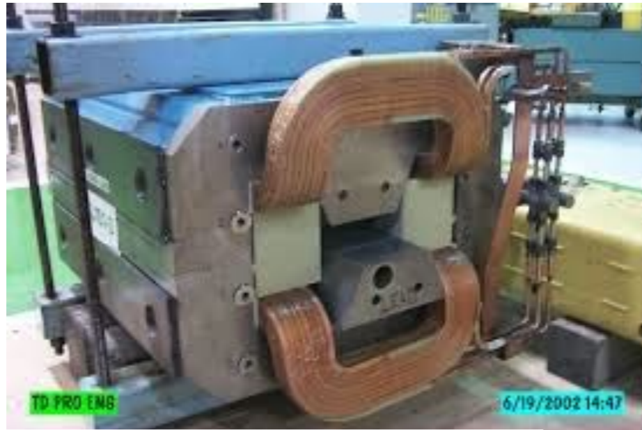
Dipole Magnet, Fermilab
