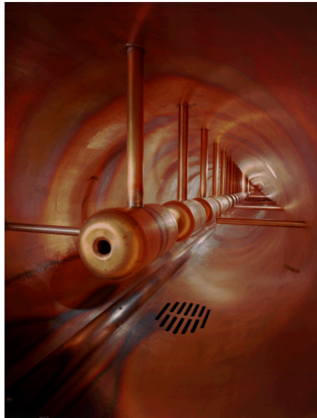
DTL tank - Fermilab
