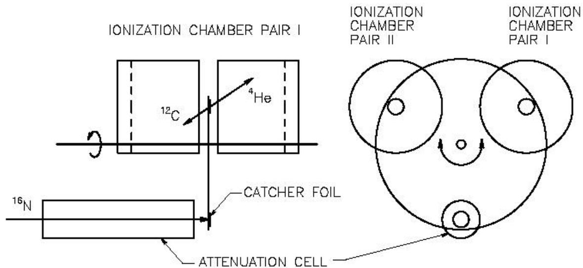
Fig. I-1. Schematic of the experimental setup used to study the beta-delayed alpha decay of  $^{16}\text{N}$ .
