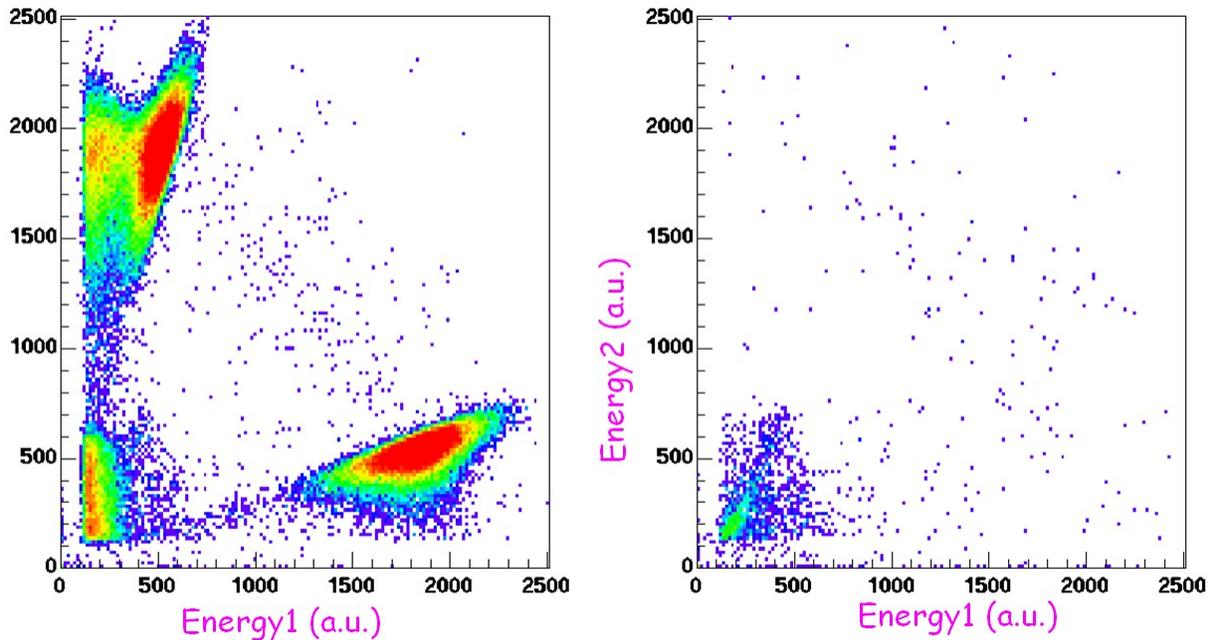
Fig. I-2. Left:  $^{12}\text{C}$ -alpha coincidences measured in one detector pair using a 10 microg/cm<sup>2</sup> thick carbon foil which was bombarded by  $^{16}\text{N}$  particles. Right: coincidence spectrum measured in the same detector pair with a non-irradiated carbon foil.
