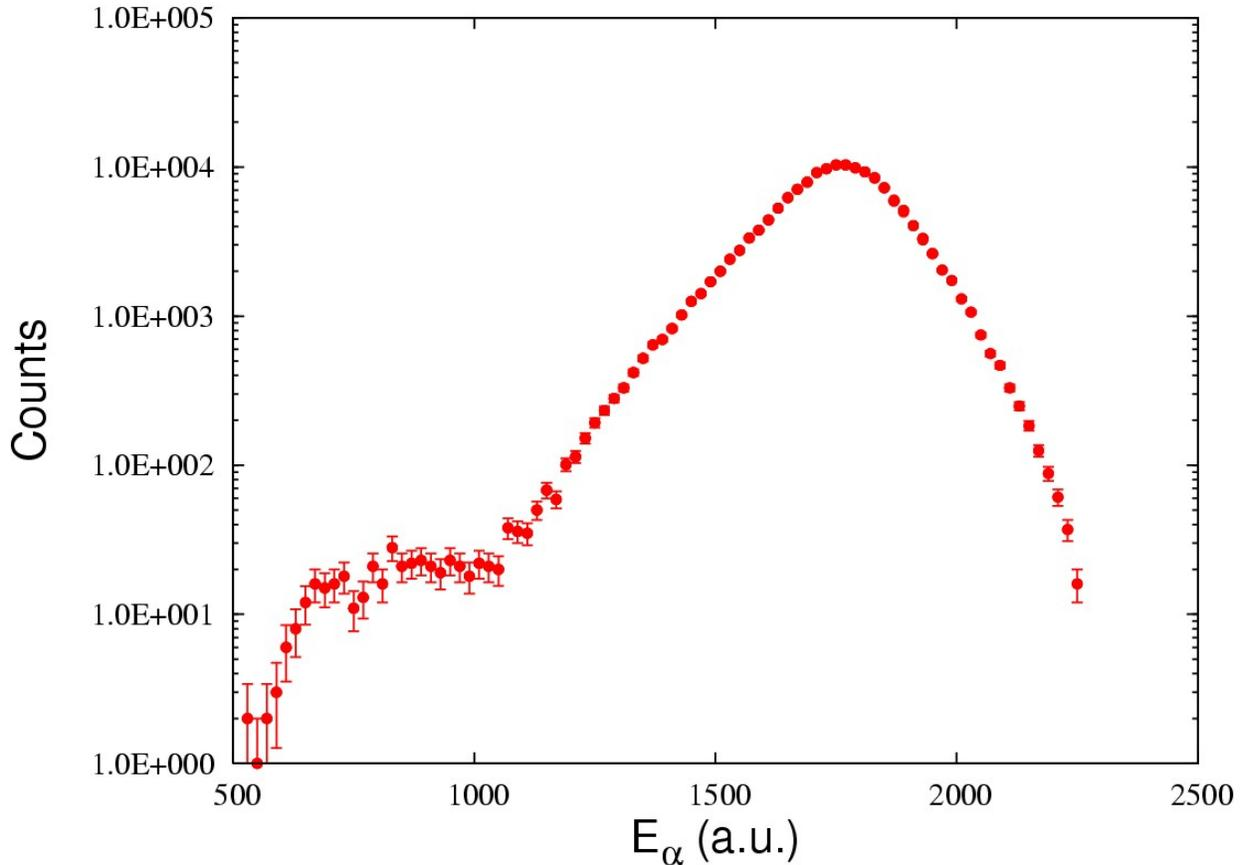
Fig. 1-3. Preliminary beta-delayed alpha spectrum from  $^{16}\text{N}$  obtained in a first experiment. This spectrum, taken at a pressure of 150 Torr has not been unfolded for the detector response.
