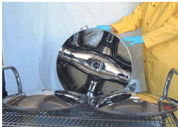
Fig. III-2. Niobium elements of the prototype \beta = 0.64 triple-spoke cavity after electropolishing and before the final closure welds.
