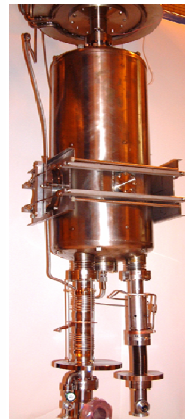
Fig. III-5. Prototype 109 MHz quarter-wave cavity for the ATLAS upgrade and for the RIA driver linac. The cavity is shown with the RF power coupler and slow-tuner yoke assembled for cold-testing. In initial cold-tests the prototype cavity could provide as much as 3 MV of accelerating potential in cw operation at 4.2 K.
