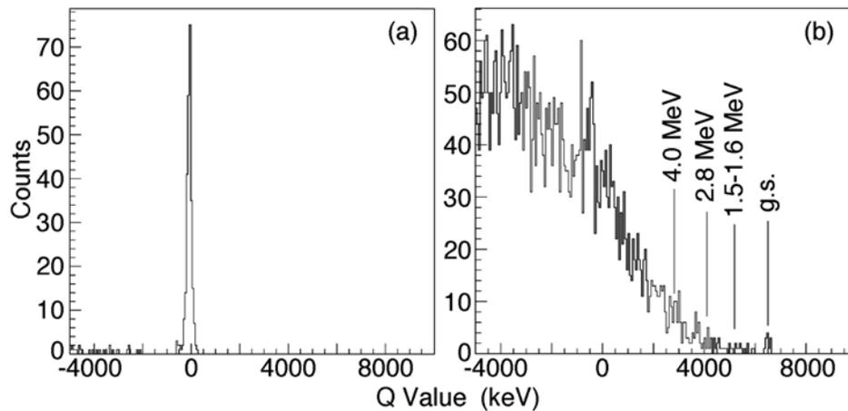
Fig. I-3. (a) Q-Value spectrum for  $^{11}\text{C} + ^{197}\text{Au}$  elastic scattering. (b) Q-Value spectrum for the  $^{12}\text{C}(^{11}\text{C},\alpha)^{19}\text{Ne}$  reaction. The vertical lines indicate the positions of various groups of excited states in  $^{19}\text{Ne}$ .
