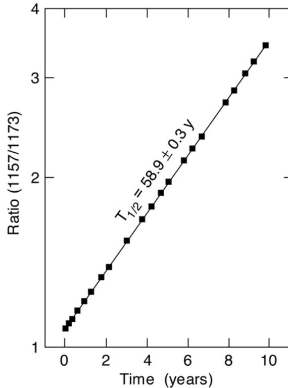
Fig. I-7. Semilogarithmic plot of the ratio of counts in the 1157-keV peak of  $^{44}\text{Ti}$  and 1173-keV peak of  $^{60}\text{Co}$  against decay time. The measurements were performed at ANL using a mixed source of  $^{44}\text{Ti}$  and  $^{60}\text{Co}$ .
