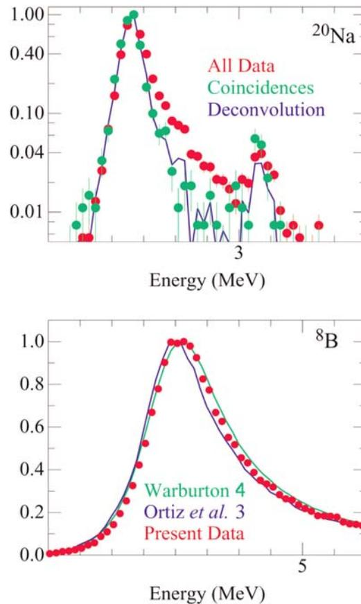
Fig. I-1. (a) Alpha calibration spectrum from the decay of  $^{20}\text{Na}$  nuclei, implanted into a  $91\ \mu\text{m}$  thick Si detector. The solid line corresponds to the deconvolution of the singles data. (b) Alpha spectrum measured from the decay of implanted  $^8\text{B}$  nuclei, compared to previous measurements (3,4).
