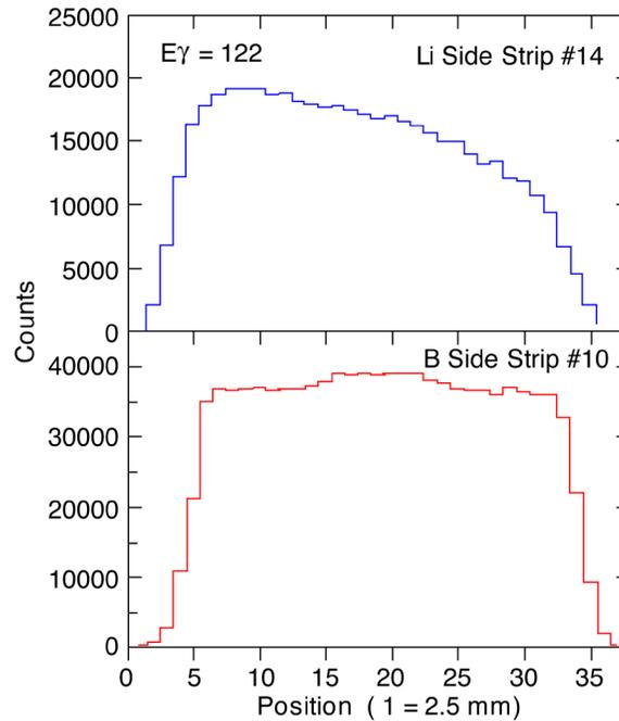
Fig. I-83. A scan along the middle of central Li and B strips using  $^{57}\text{Co}$  122-keV  $\gamma$  rays to measure efficiency. The fall-off on the Li side was remedied on the second prototype counter.
