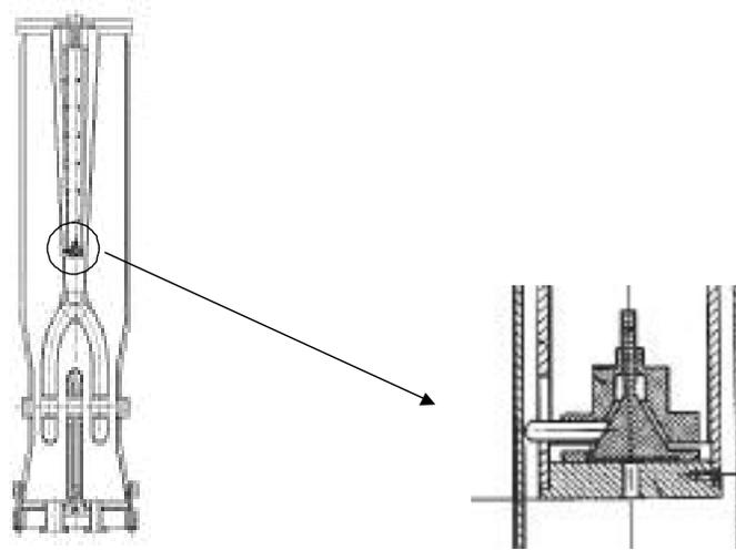
Figure II-3. Components of the Vibration Damper
