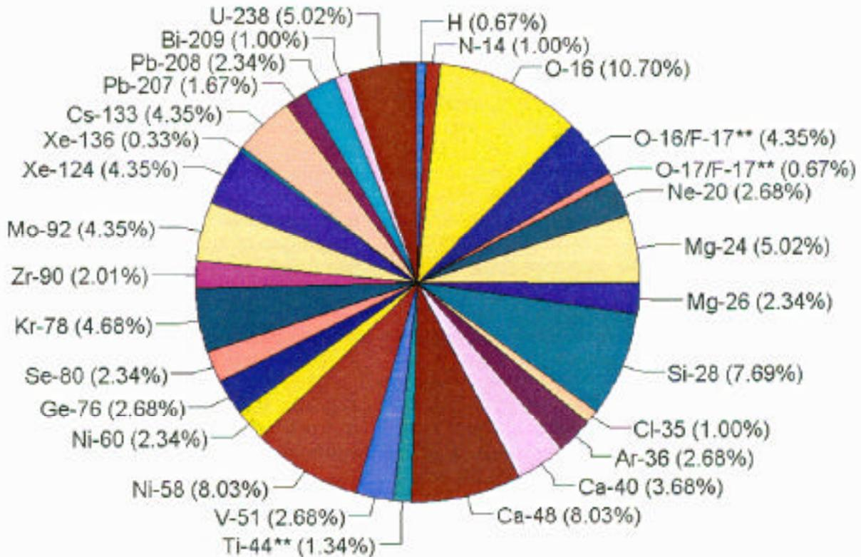
Figure II-1. Distribution of beam time, by isotope, provided by ATLAS in FY1999. A total of 29 different isotopes were provided to the research program. Radioactive beams of  $^{17}\text{F}$  and  $^{44}\text{Ti}$  comprised 6.4% of all beam time in FY1999.
