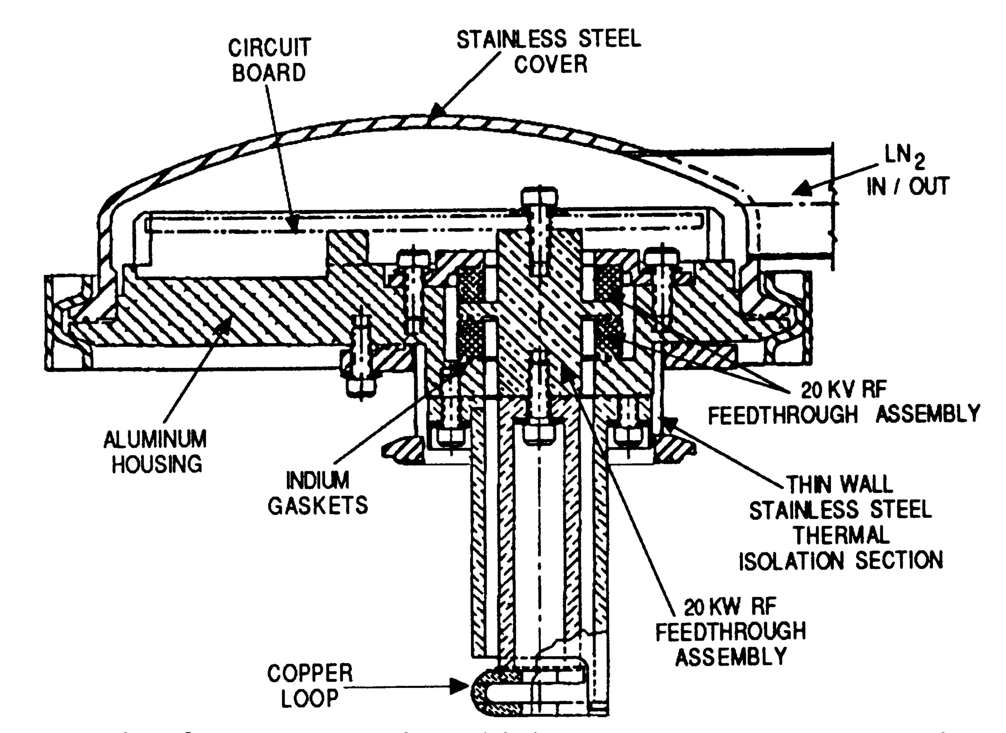
Fig. 2. The fast-tuner unit, which operates at 77 K. The copper loop projects into the superconducting cavity, and can couple as much as 30 KVA of reactive power into the tuner. The overall diameter is approximately six inches.
