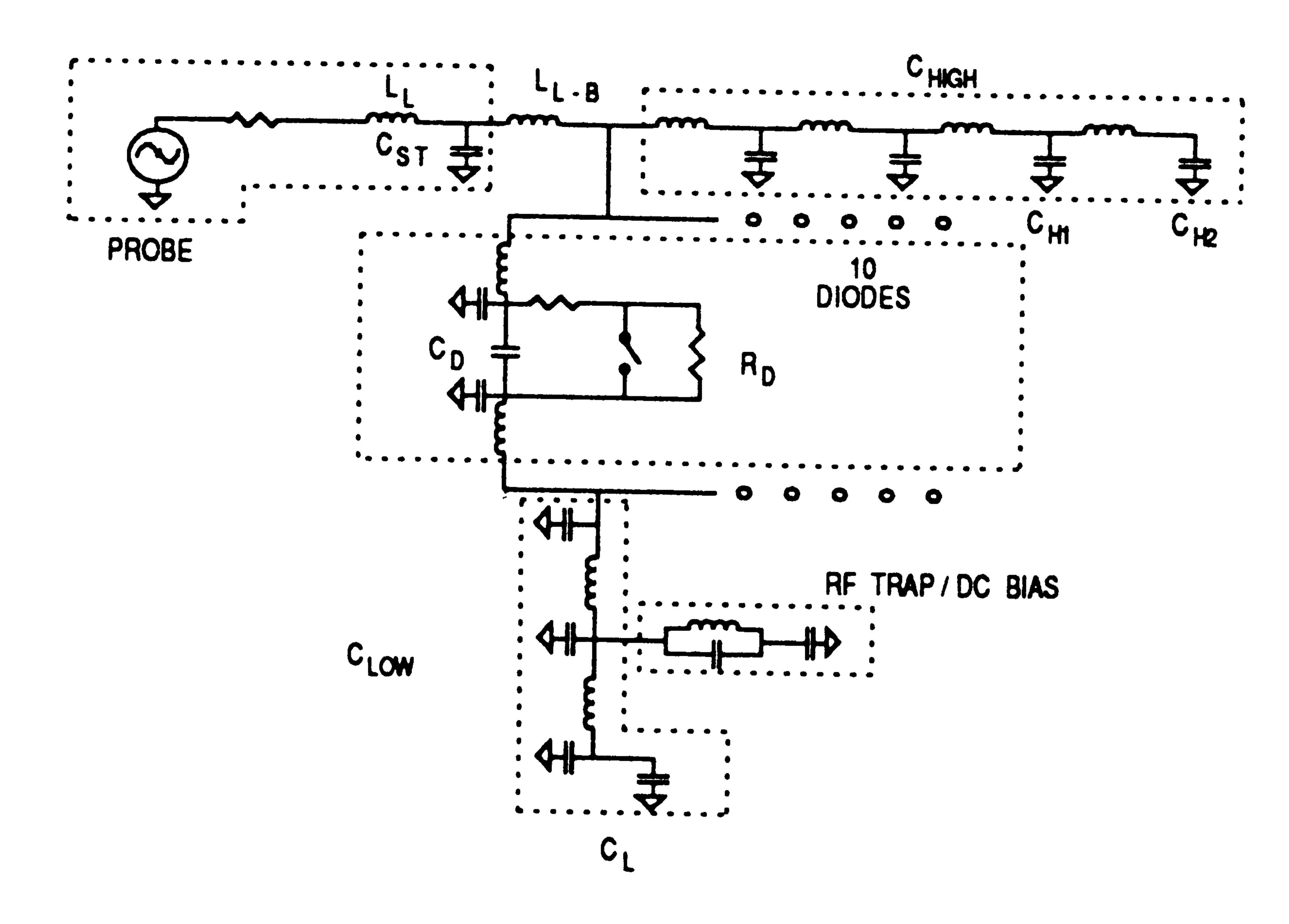
Fig. 1. Equivalent circuit model for the fast-tuner. Components modeling one of ten PIN diodes are shown.
