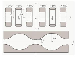
Figure 1: ARF and RFQ channels.
