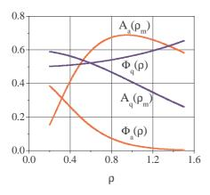
Figure 2: Accelerating gradients and form-factors as a function of unitless aperture,  $\rho_m$ , and radius,  $\rho$ .
