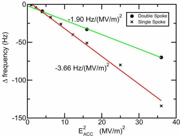
Figure 5 Static field Lorentz force detuning for the single spoke cavity (crosses) and the two-cell spoke cavity (circles) as a function of the square of the accelerating gradient. All ports are unconstrained.
