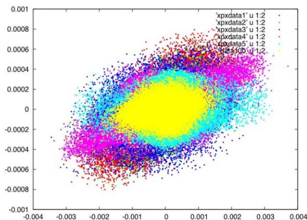
Figure 2: Transverse phase-space plot (x vs px) of 10M particle simulation for five-charge-state uranium beam at the exit of linac for the ANL RIA design. As described in the text, the plotting algorithm displays all the halo particles. The dense central region is obtained by plotting every 100<sup>th</sup> particle.
