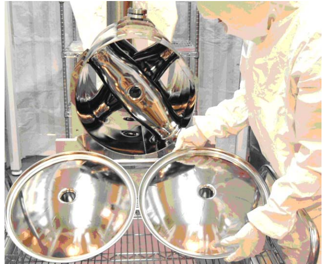
Figure 2: Niobium elements of the prototype superconducting \beta_G=0.50 triple-spoke cavity after electropolishing and just prior to welding the complete assembly.
