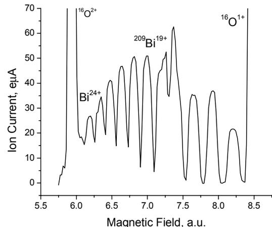
Figure 2: Bismuth beam intensities at different charge states.
