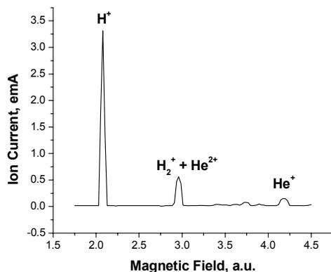
Figure 4: Hydrogen beam intensities.
