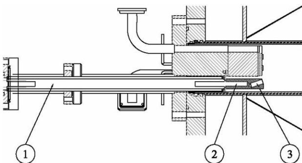
Figure 1: BIE-100 with (1) oven support assembly, (2) cartridge heater insertion point and (3) sample material.
