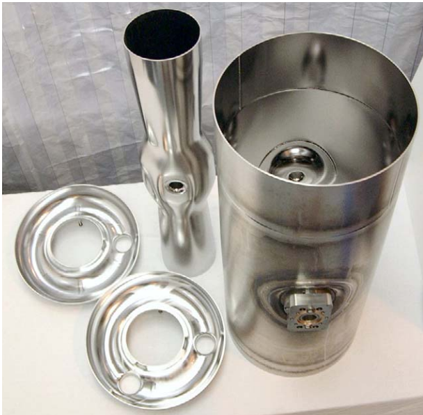
Figure 2: Electropolished niobium components of the RIA half-wave cavity.
