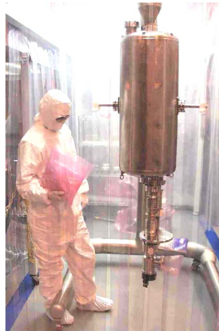
Figure 3: Clean room assembly of the HWR together with a variable coupler and pumping system.
